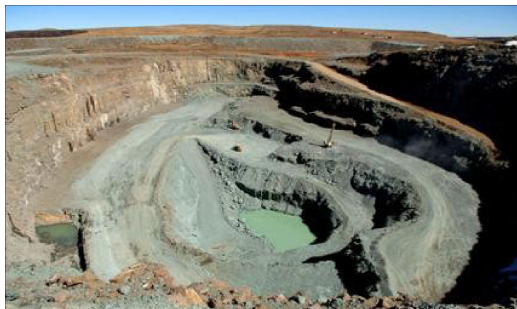
A view of the Letseng satellite pit. The gray material is kimberlite, whose dykes and pipes host the diamond crystals. (Photo courtesy Gem Diamonds)
